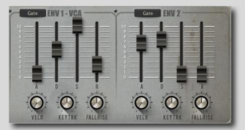
*ENV 1 – VCA* is labeled *VCA* because it is hardwired to the Voltage Controlled Amplifier and it's the envelope for controlling the volume of the synth. However, it can be used to modulate other parameters as well.
