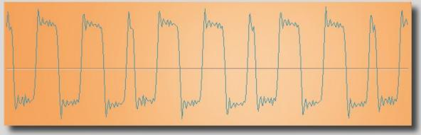
An example of the resulting (slave) pulse wave with a duty cycle of 50%
