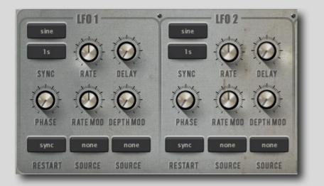
*Tyrell*'s LFO (Low Frequency Oscillator) section features two identical LFOs that are used as modulation sources. *LFO 1* is "hardwired" to the vibrato function.
