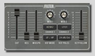
*Tyrell Nexus 6* features a self-oscillating multimode filter with a unique *Mixspr* (mixspread) function.
