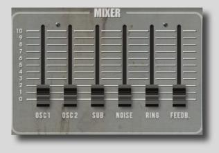
The *Mixer* is very straight forward. It controls the volume of the six elements going through it and the amount of each going into the filter.
