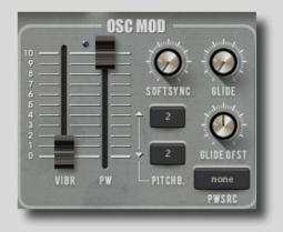
The oscillator modulation section (*OSC MOD*) consists of the following controls...
